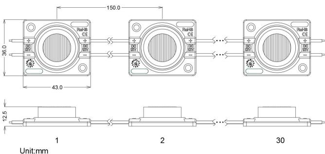
Note: the pitch based on 120mm
