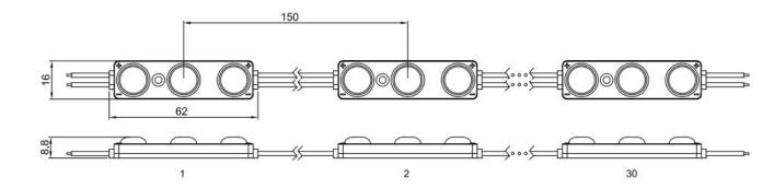
unit:mm Note:the pitch based on 150mm wire
